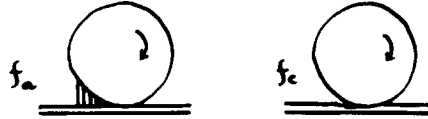
Fig. 2. Rolling friction caused by adhesion ( f_a ) and that caused by compressive deformation of the substrate ( f_c ).
